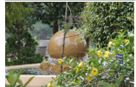
Fountain: This granite ball is about 4' in diameter and is floating on water being pumped from underneath.
